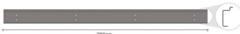
PERFIL LATERAL DA CARRETA PARA ASSOALHO DE FERRO SP389 - 2965mm - ch. 4,25mm - 25,700kg SP389A - 2225mm - ch. 4,25mm - 18,000kg SP389B - 2430mm - ch. 4,25mm - 19,720kg SP389C - 2325mm - ch. 4,25mm - 19,600kg
