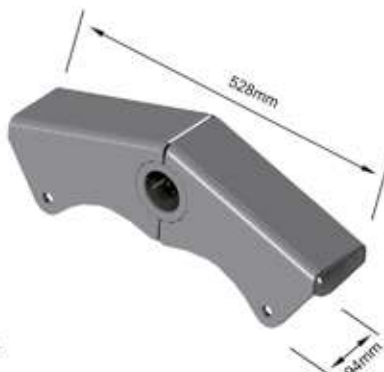
BALANÇA ASA DELTA ESTAMPADA P/PINO Ø 61,30mm P/CARRETA 2012 SP535 - ch. 6,35mm
