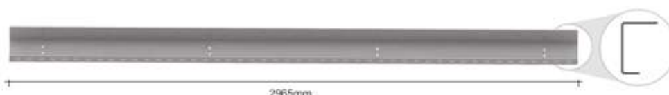
PERFIL LATERAL DA CARRETA COM FURAÇÃO SP372 - 2965mm - ch. 4,25mm - 25,000kg SP372A - 2225mm - ch. 4,25mm - 18,760kg SP372B - 2430mm - ch. 4,25mm - 20,440kg SP372C - 2325mm - ch. 4,25mm - 19,600kg
